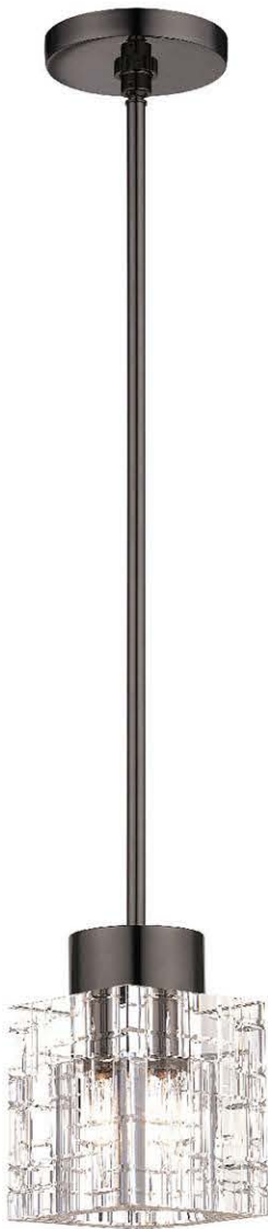
46181-46 4.75" CRYSTAL PENDANT 5" DIA 15.25" - 81.25" ADJ.H WIRE 12' CANOPY 5" DIA 0.75" H CRYSTAL SHADE 4.75" SQ 5.5" H MAX WATT 1 - 60W CAND BASE INCLUDES 6" 12" 3 - 18" STEM SECTIONS ACCOMMODATES SLOPED CEILINGS BULB OPTIONS \varnothing B10
